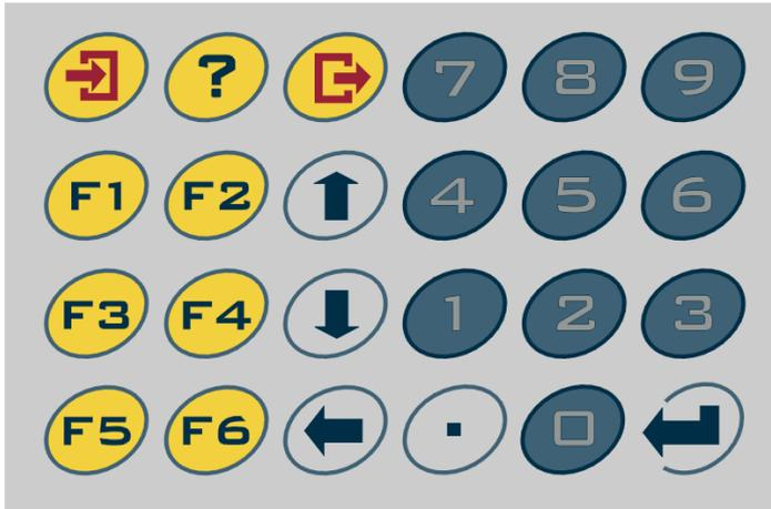
The keyboard gives no mechanical feedback, you can't feel if a key is closed or not. Instead you hear a short beep to give the user an indication if the key is pressed or not.
