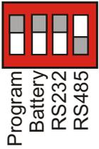
Set the DIP switch to ON,ON,ON,OFF.
