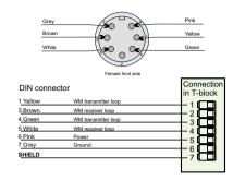
Step 3: You must remove the 2 jumpers because we connect a power supply to the t-blok.
