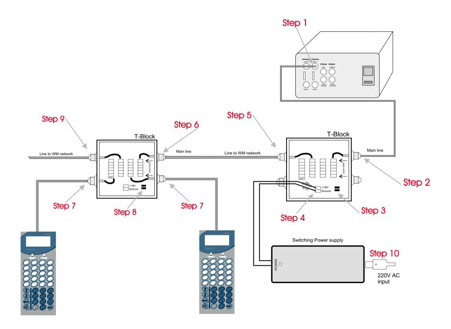
Step 1: Connect the cable with connector (see pic.) to the concentrator.
